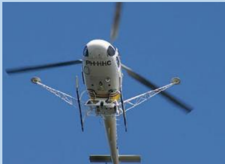
Aerial LiDAR Survey at 40 scans per metre
