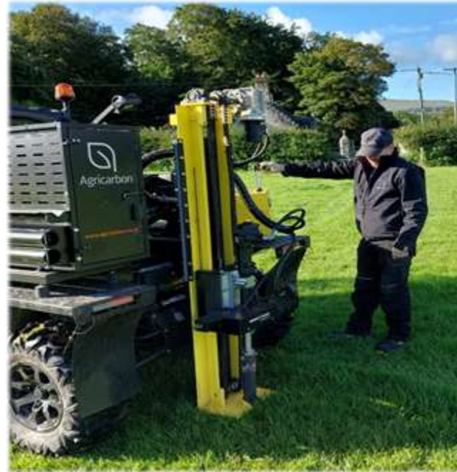
Soil Sampling to one metre deep
