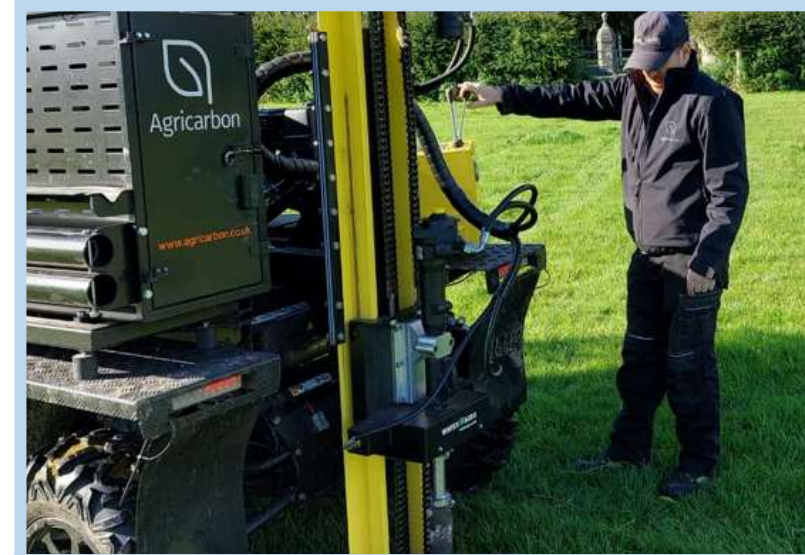
Soil Sampling to one metre deep
