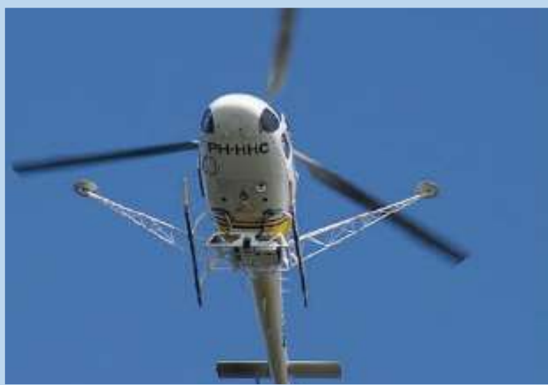
Aerial LiDAR Survey at 40 scans per metre
