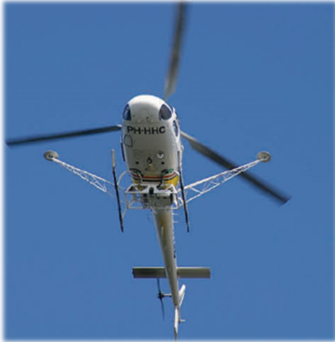
Aerial LiDAR Survey at 40 scans per metre
