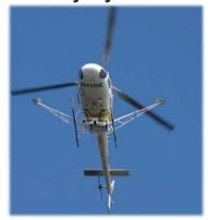
Aerial LiDAR Survey at 15 scans per metre
